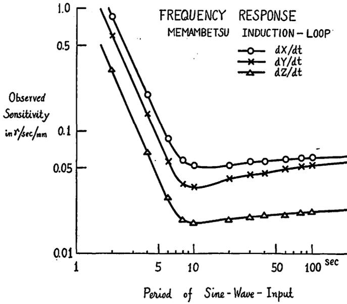
Fig. 5. (b) Sensitivities of the induction magnetograph at Memambetsu.
