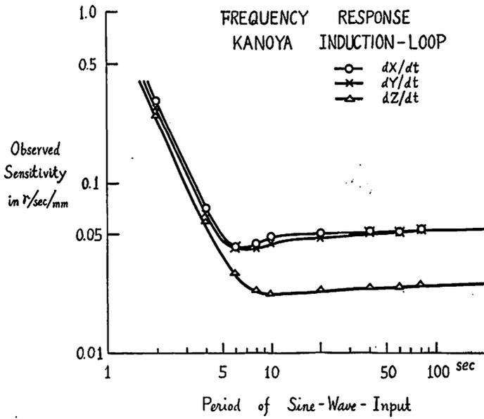
Fig. 5. (c) Sensitivities of the induction magnetograph at Kanoya.
