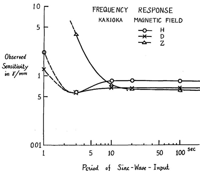
Fig. 5. (a) Sensitivities of the quick-run magnetograph at Kakioka.
