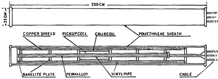
Fig. 1 The antenna of ELF (loop-antenna).
