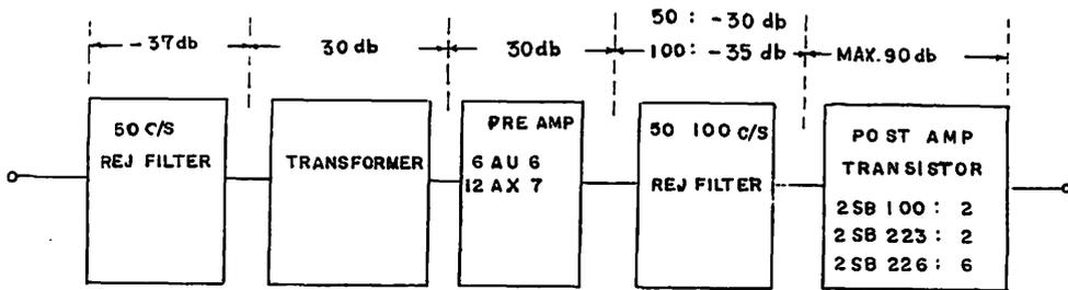
Fig. 5 The block diagram of the amplifier and its' gain for loop-antenna.
