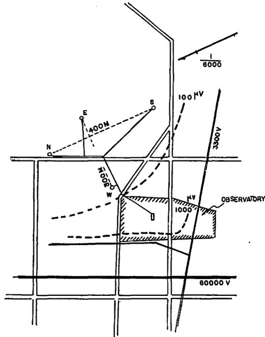
Fig. 9 The plan of the Memambetsu observatory and its neighborhood, and the distribution of 50 cps noise.
