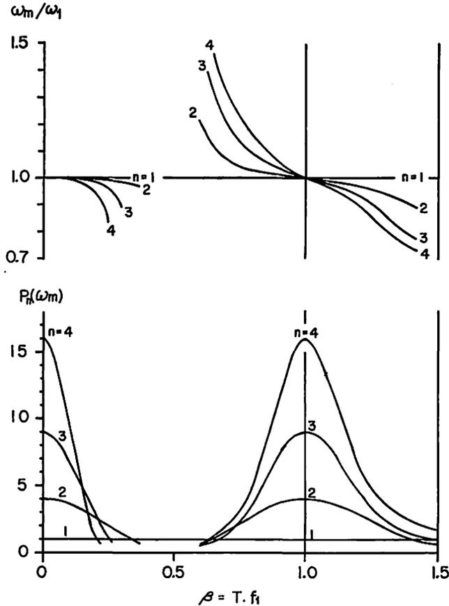
Fig. 5 Variations of maximum power  $P_n(\omega_m)$  and the corresponding frequency  $\omega_m$  with respect to  $\beta = T \cdot f_1$ .
