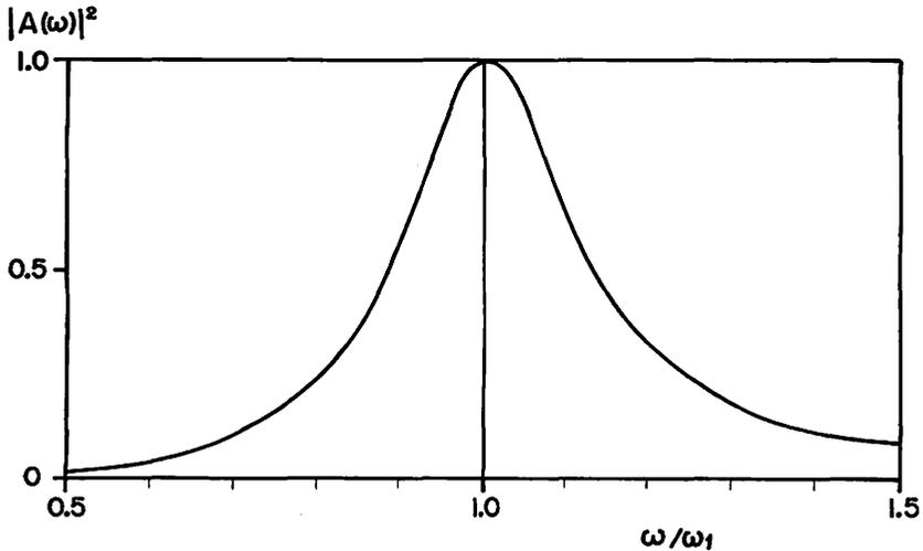
Fig. 4 Frequency response function  $|A(\omega)|^2$  of the earth-ionosphere cavity.
