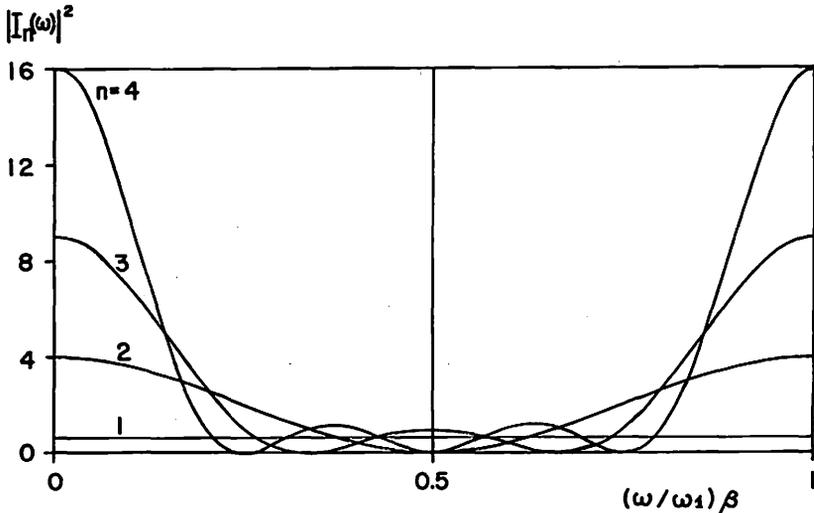
Fig. 3 Excitation  $|I_n(\omega)|^2$  by multiple strokes.  $n$  is the number of stroke and  $\omega_1$  is the first Schumann resonance frequency.  $\beta = T \cdot \omega_1 / 2\pi$ .
