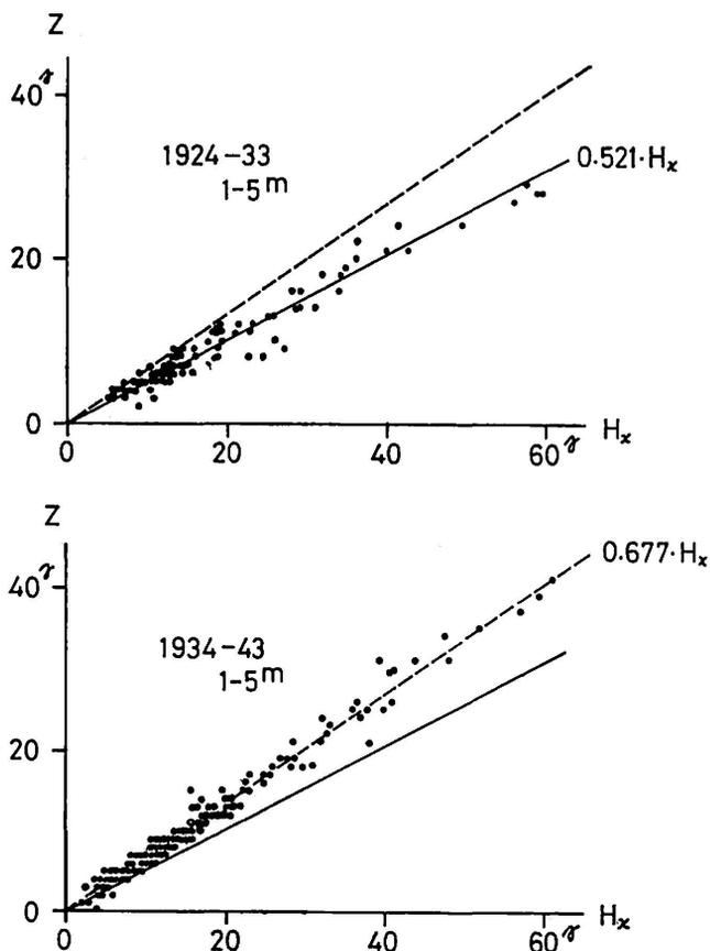
Fig. 3 Mean slope of the plane in which vectors of geomagnetic variation are confined at Kakioka for 1924-33 (full line) and for 1934-43 (broken line). Each dot represents the observed one where  $Z$  is the vertical component and  $H_x$  the horizontal component in the direction of the normal of the plane.
