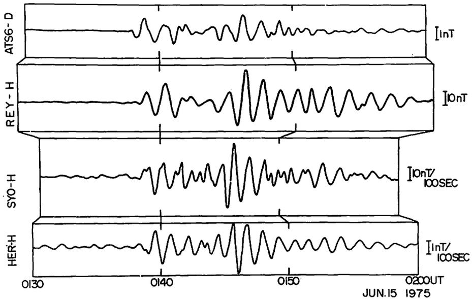
Fig. 2. Simultaneous appearance of *Pi2* event at ATS 6 and at the ground based stations. Two substorm onsets started at 0139 and 0145 UT. The wave trains are illustrated with D (east-west) component for the data in the magnetosphere, while illustrated with H (north-south) component for the data on the ground.
