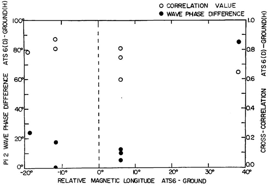
Fig. 7.  $Pi2$  wave-phase difference between the D (east-west) component at ATS 6 and the H (north-south) component on the ground (solid circle), and the maximum cross-correlation value derived from the cross-correlation function (open circle).
