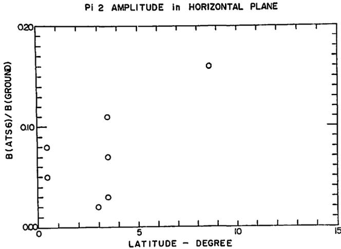
Fig. 4. Ratios of the  $Pi2$  wave amplitude at ATS 6 to that at the conjugate ground-based stations (Syowa Station or Reykjavik) are plotted as a function of the relative latitude of ATS 6 to the geomagnetic equatorial plane.
