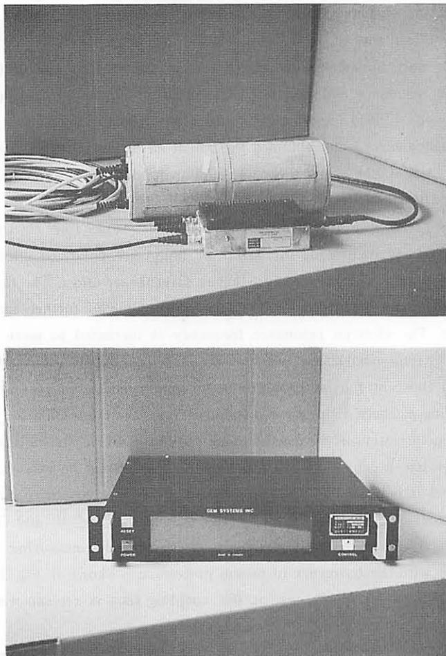
Fig. 10 Overhauser magnetometer; Sensor unit (upper) and amplifier unit (lower).
