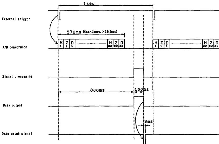
Fig. 7 Timing chart of A / D conversion of the fluxgate magnetometer.
