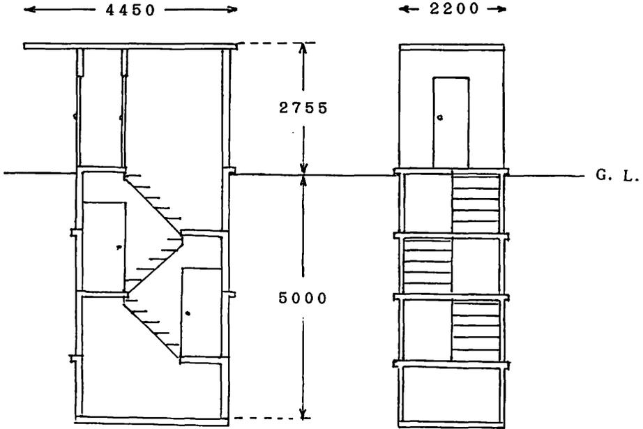
Fig. 8 The sensor house for the fluxgate magnetometer.
