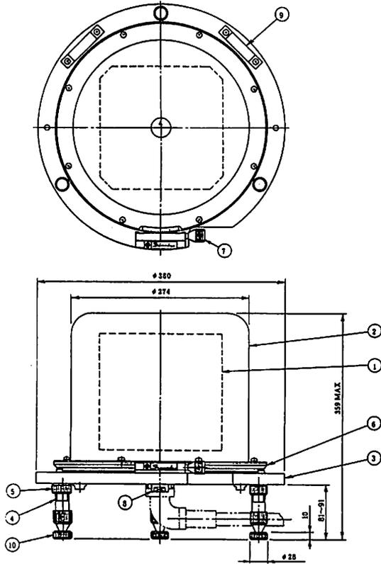
Fig. 5 Sensor unit of the fluxgate magnetometer.
