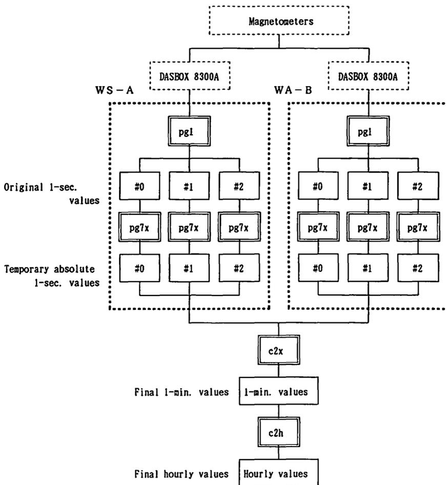
Fig. 21 Flow of the data processing. Hardwares, data files and corresponding programs are in dashed, solid and double squares, respectively.
