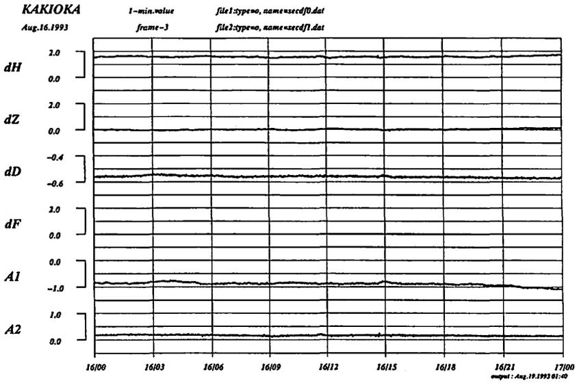
Fig. 22(b) Differences between two magnetometers (dH, dZ, dD) and A-values ( $F - (H^2 + Z^2)^{1/2}$ ) for trigonometric check. A1 is for the fluxgate and A2 for Overhauser magnetometers.
