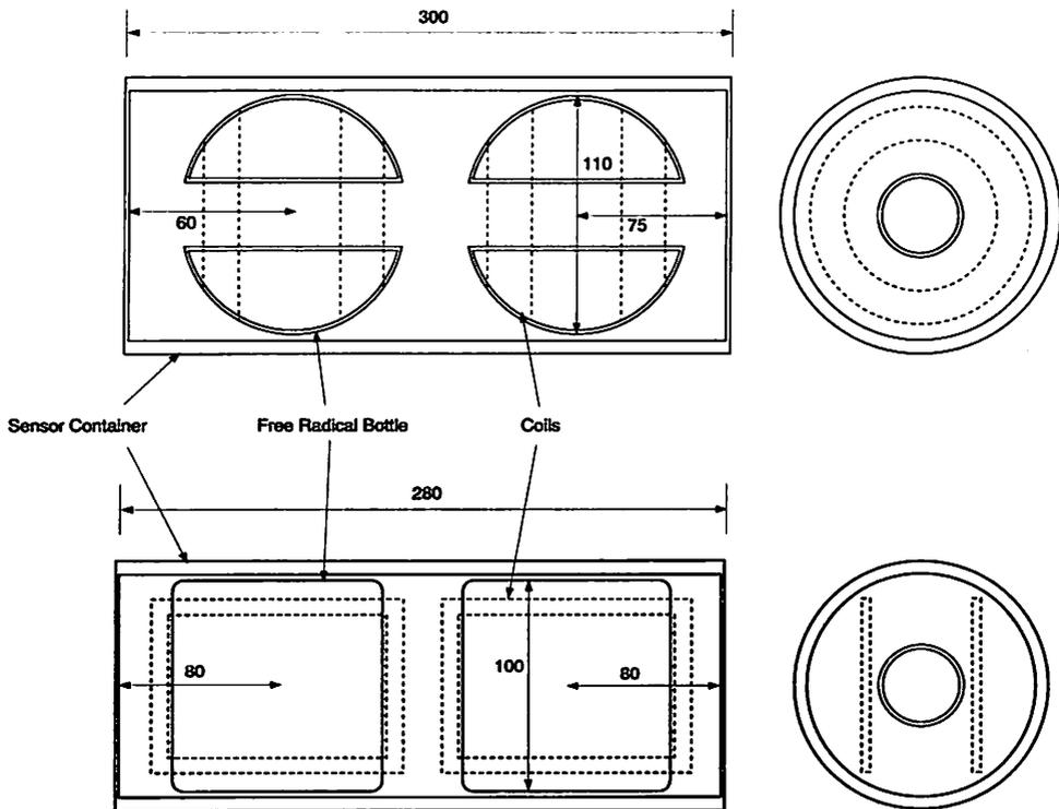
Fig. 12 Sensor design of Overhauser magnetometer; component observation (upper) and total intensity observation (lower).
