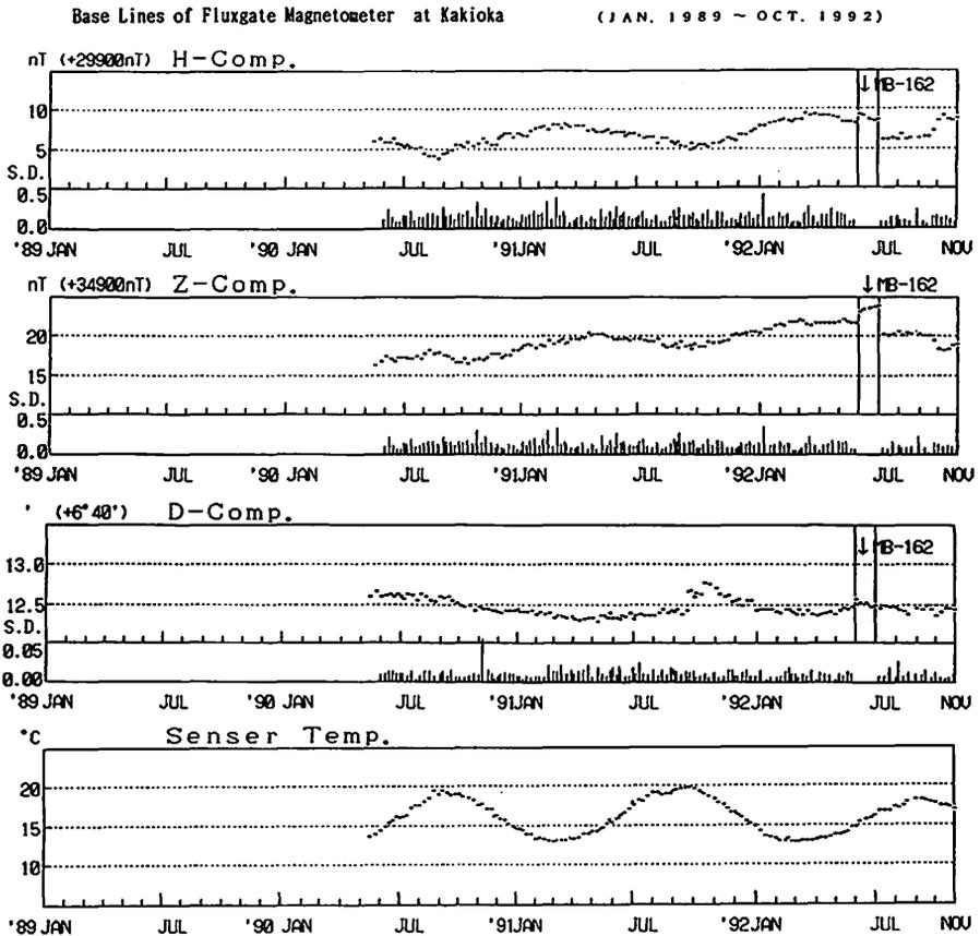
Fig. 9 Base lines of the fluxgate magnetometer (1990 May - 1992 Oct.) obtained by the routine observation.
