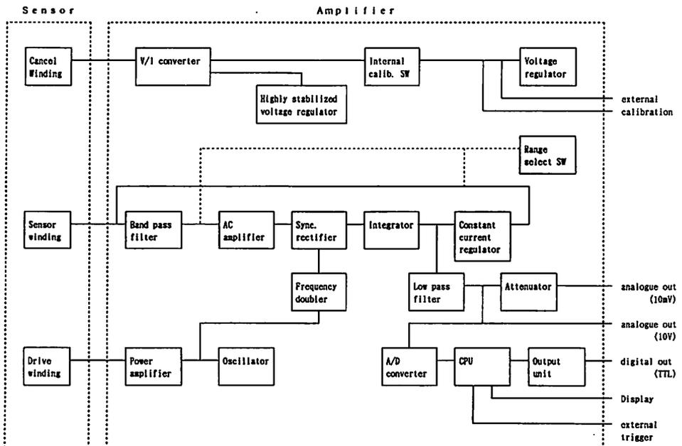
Fig. 6 Block diagram of the measurement circuit of the fluxgate magnetometer.
