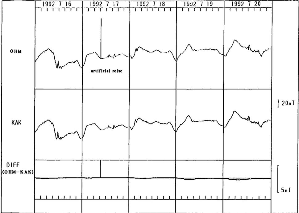
Fig. 15(a) Comparison of H component observation of Overhauser magnetometer (OHM) with KASMMER (KAK) and difference (DIFF).
