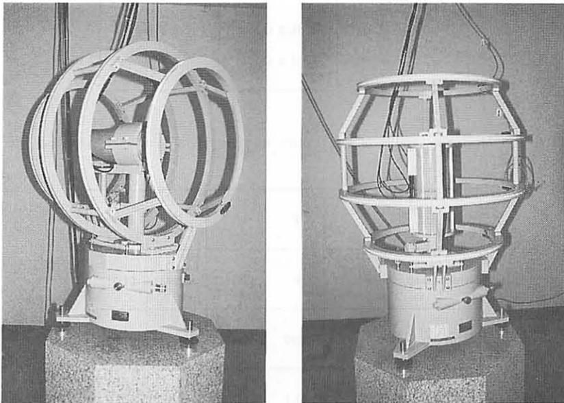
Fig. 14 Fanselau-Braunbek coils; for Z and Hyz measurements (left) and for H measurement (right).
