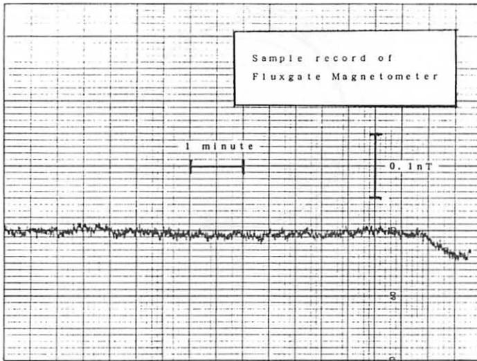
Fig. 3 Test sample of analogue record of magnetic observation by the adopted sensor core for the fluxgate magnetometer.
