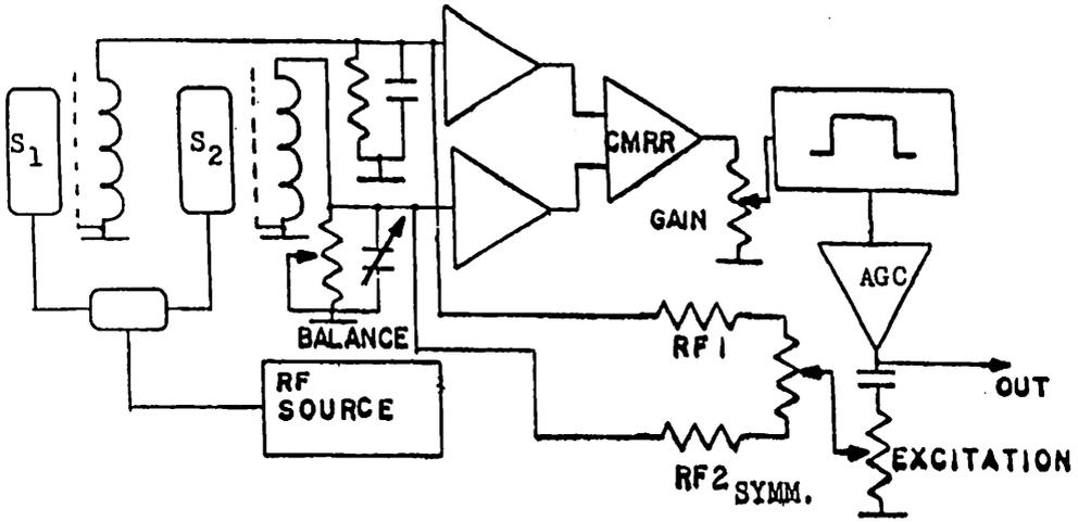
Fig. 11 Block diagram of Overhauser magnetometer measurement circuit.
