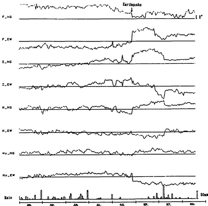
Fig. 16 Long term variations of the tilting of the pillars of the optical pumping magnetometers.
