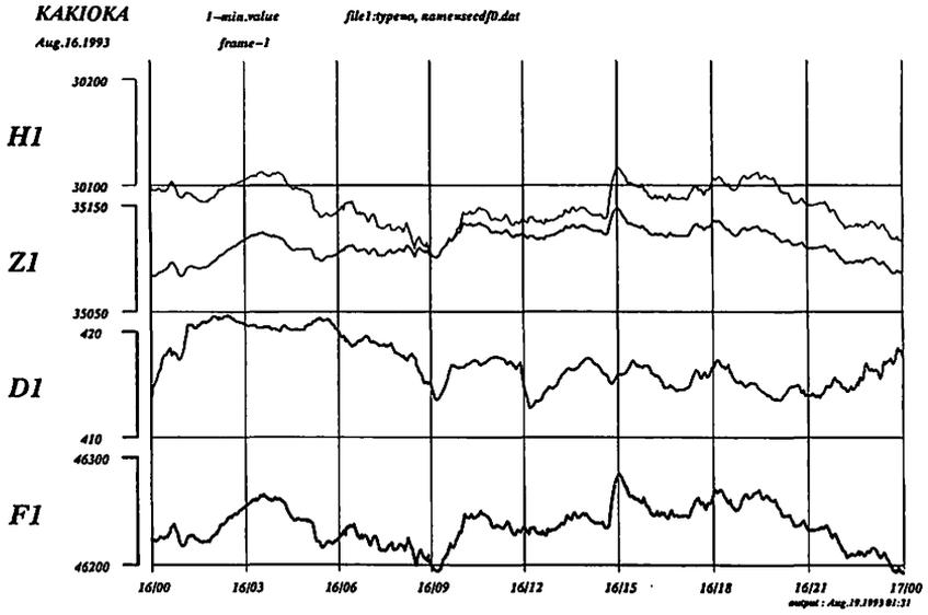
Fig. 22(a) Original data of the fluxgate magnetometers.
