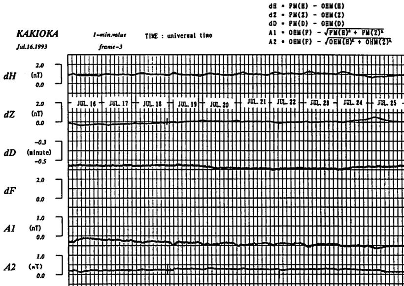
Fig. 23 Comparison of component observations of Overhauser magnetometers, OHM (H), OHM (Z), OHM (D), OHM (Z) and those of the fluxgate magnetometer, FM (H), FM (Z), FM (D).
