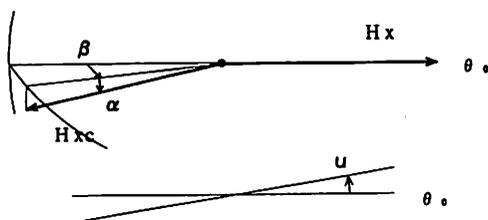
Fig.13 Mechanical errors ( $\alpha, \beta$ ) of the compensating coil and coil level ( $u$ ) for the D component measurement.
