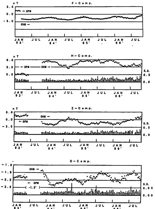
Fig.14 Observed base line values of F, H, Z and D components by OHMs (OCT. 1993 - OCT. 1996). S.D. means the standard deviation of each absolute observation.
