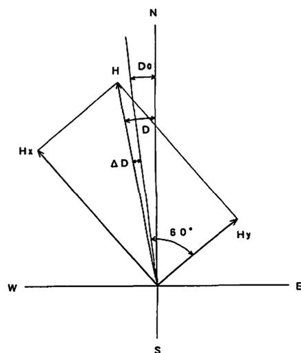
Fig. 1 Principle of the D component measurement using the optical pumping magnetometer.
