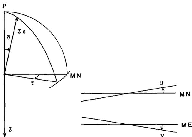
Fig.11 Mechanical errors ( $\eta, \tau$ ) of the compensating coil and coil level ( $u, v$ ) for the H component measurement.
