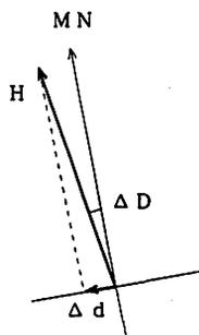
Fig. 5 Relation between  $\Delta D$  and  $\Delta d$ . MN means magnetic north (mean magnetic meridian).
