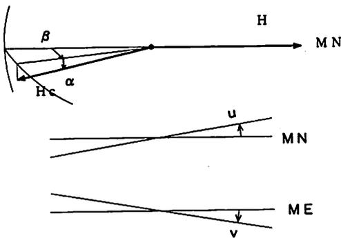
Fig.12 Mechanical errors ( $\alpha, \beta$ ) of the compensating coil and coil level ( $u, v$ ) for the Z component measurement.
