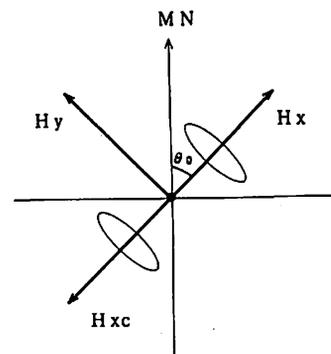
Fig. 6 Direction of the horizontal coil axis for the D component measurement and  $H_x$ ,  $H_y$  component.
