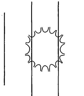
Fig. 2 Zone of the uniformity less than  $10^{-4}$  in the Fanselau-Braunbek coil. The calculated magnetic field is in the direction of the coil axis.
