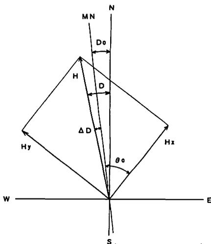
Fig. 8 Relation between the  $H_x$ , H and D component.
