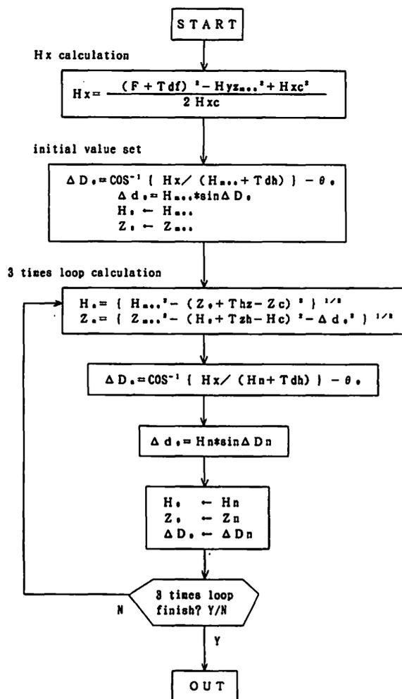
Fig.10 Calculating procedure for the components measurement with OHMs.
