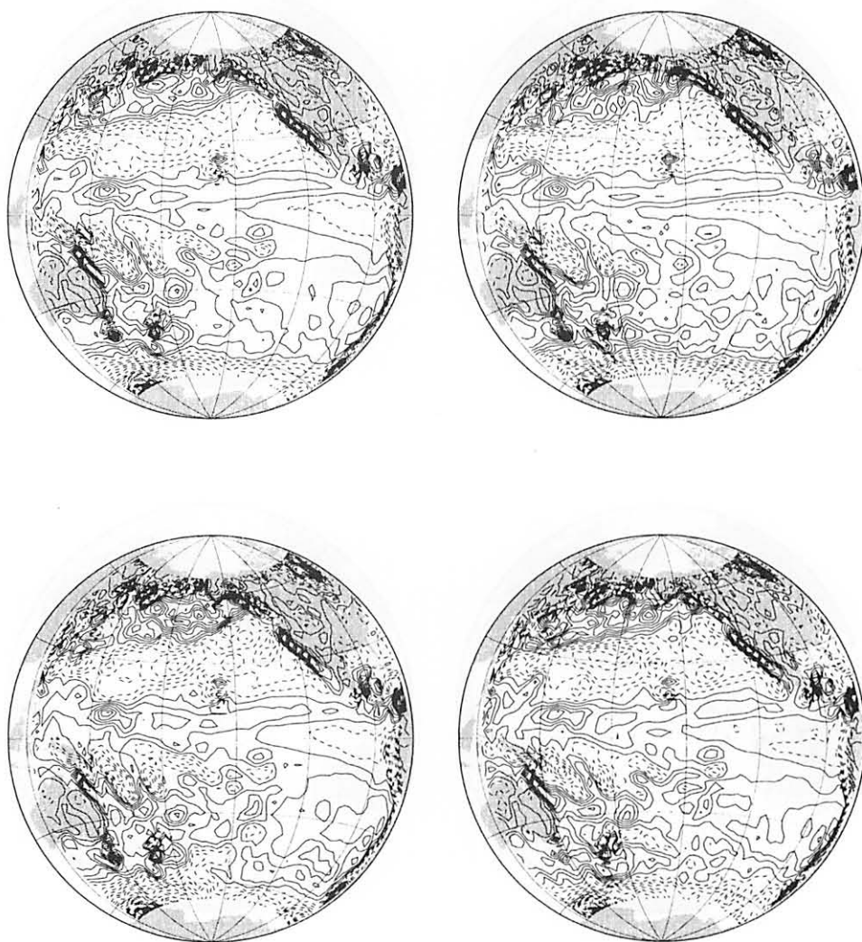
Figure 63: Mean of the curl for 3.6 years and each year clockwise from the top left corner. Contour lines are drawn every 2 \times 10^{-9} \text{ g/cm}^2 \text{ s}^2 with dotted (negative values) and solid (positive values) lines.
