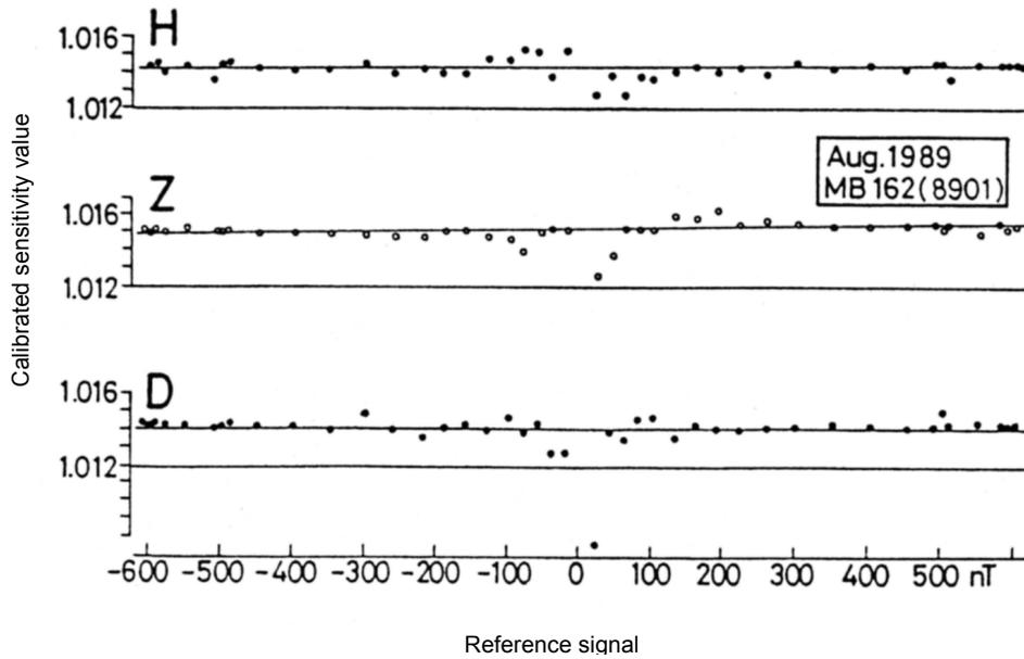
Fig. 3 Linearity of sensitivity values of the fluxgate magnetometer
