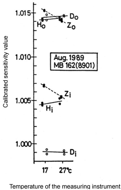
Fig. 5 Dependence of the calibrated sensitivity value on temperatures
