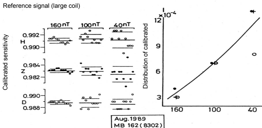
Fig. 2 Reliability of the calibrated sensitivity value (the state of distribution of repeatedly measured values and the strength of a reference signal)
