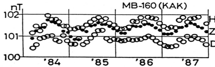
Fig. 1 Change in the sensitivity of the fluxgate magnetometer (change in the output relative to the built-in reference signal of 100 nT)
