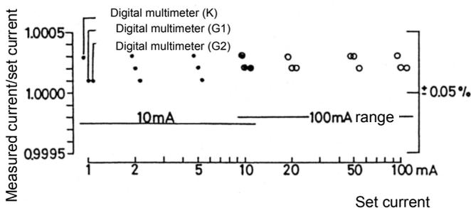
Fig. 6 Accuracy of the current used to form a reference magnetic field (type 2561)
