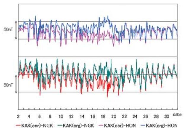
Fig. 4 Hourly values of the H component of the geomagnetic field - differences between the values at Kakioka (KAK), Honolulu (HON) and Niemegek (NGK) (Aug. 2 to 31, 1933).
