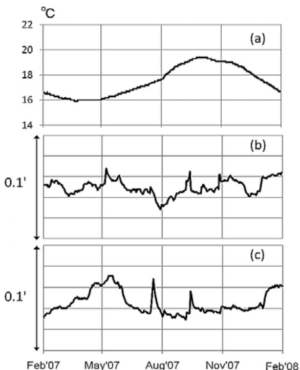
Fig. 2 Changes in inclination and temperature using a high-sensitivity triaxial fluxgate magnetometer at KMO (from Feb. 1, 2007 to Jan. 31, 2008) (a) shows the temperature data, (b) tilt (north-south), and (c) tilt (east-west). Significant tilt variations in July and September is due to heavy rainfall.
