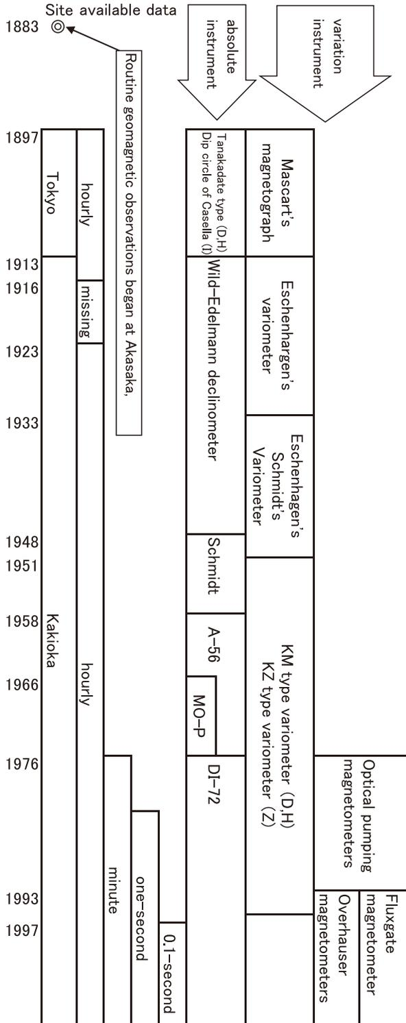
Fig. 1 Observation instruments used by CMO and KMO and the changes in available data.
