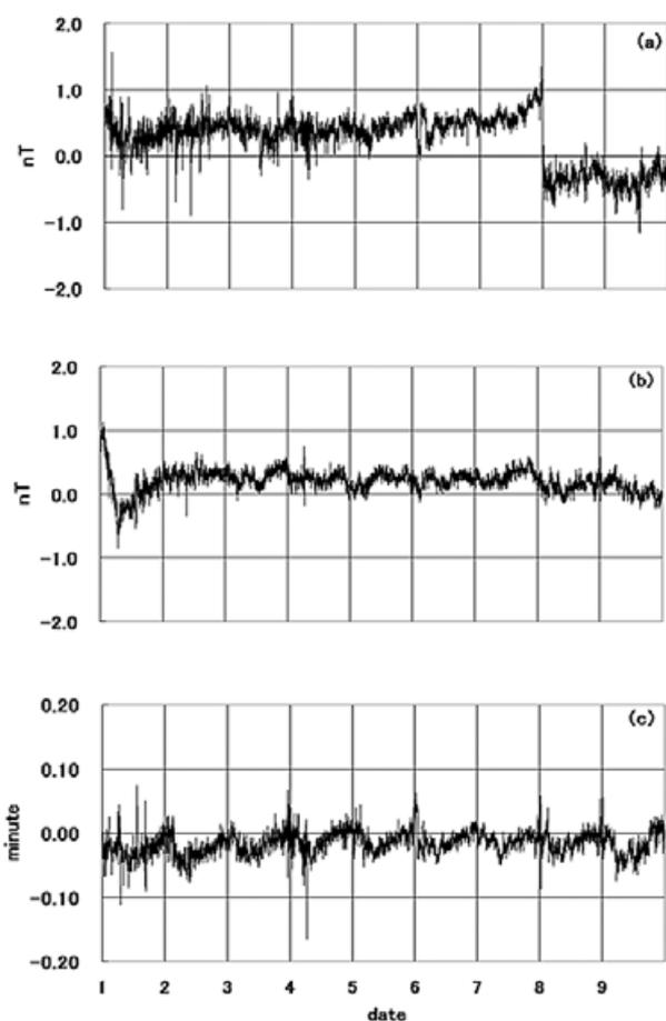
Fig. 5 Differences between the digital values obtained by an optical pumping magnetometer and the values with a one-minute resolution obtained from the bromide paper records (Aug. 1 to 9, 1984)
