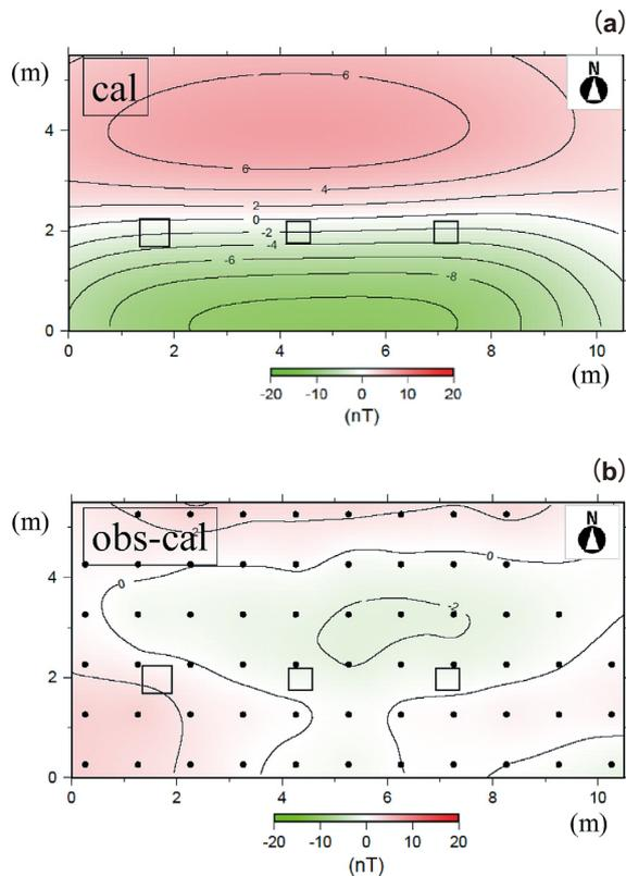
Fig. 7 (a) Total magnetic intensity profile calculated from the shape of the soil excavation area presented in Fig. 6.
