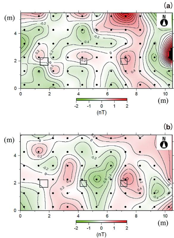
Fig.15 Profile of the differences in the total magnetic intensity in the absolute observation house measured in the first and third surveys (calculated as the third survey results - the first survey results). The contour interval is 0.2 nT.
