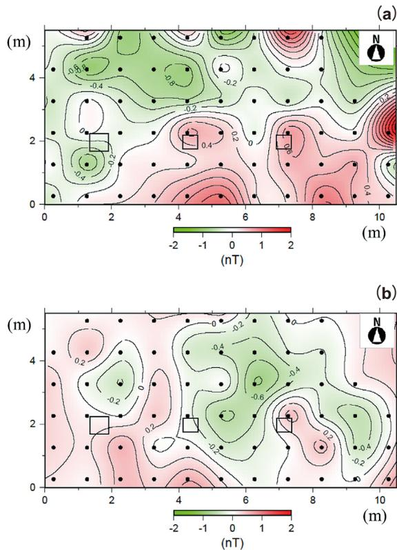
Fig.14 Profile of the differences in the total magnetic intensity in the absolute observation house measured in the first and second surveys (calculated as the second survey results - the first survey results). The contour interval is 0.2 nT.
