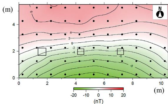
Fig. 5 Profile of the total magnetic intensity in the absolute observation house at 1.5 m above the floor after subtracting the pre-construction profile.
