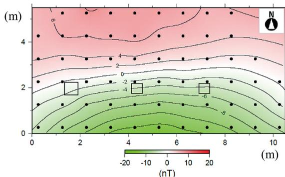
Fig. 5 Profile of the total magnetic intensity in the absolute observation house at 1.5 m above the floor after subtracting the pre-construction profile.
