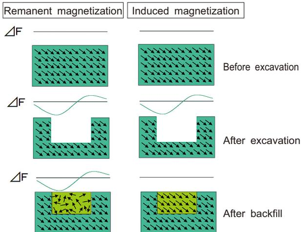
Fig. 1 Schematic diagram of the formation of magnetic anomaly due to excavation and backfill of soil.
