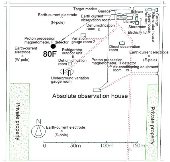
Fig. 9 Site plan of Kanoya Magnetic Observatory. The point marked 80F is the total magnetic intensity continuous observation point at Kanoya.
