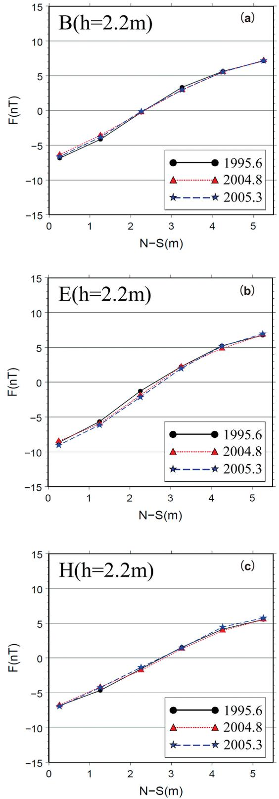
Fig.13 Total magnetic intensity measured in the absolute observation house along the north-south survey lines at 2.2 m above the floor. Black, red, and blue lines represent the first survey (June 1995), the second survey (August 2004), and the third survey (March 2005), respectively. Panels (a), (b), and (c) show measurements along survey lines B, E and H, respectively.
