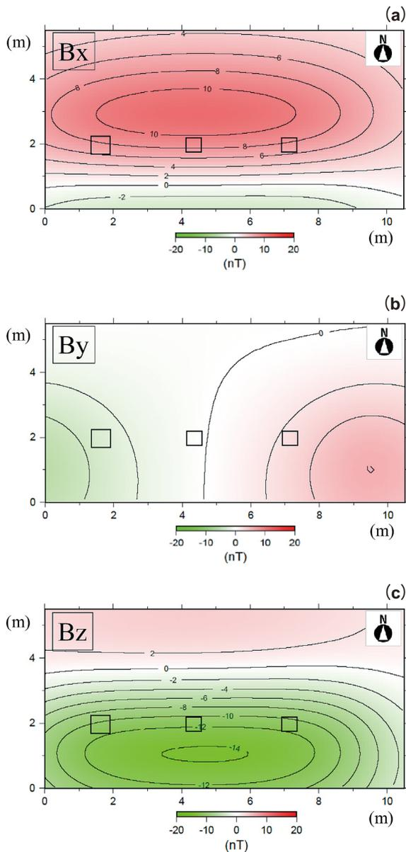
Fig. 8 Profiles of three components of magnetic field in the absolute observation house at 1.5 m above the floor as estimated by the excavation model. The contour interval is 2 nT. Panel (a): X component; Panel (b): Y component (facing east, positive); Panel (c): Z component.
