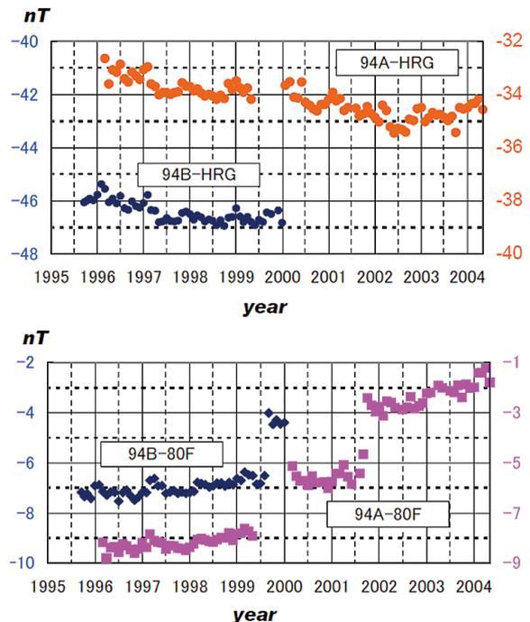
Fig.10 Changes over time in differences between the total magnetic intensity observation points 94A and 94B (in the absolute observation house), 80F and HRG. The remote comparative observatory at Haraigawa (HRG) is located 4 km northwest of Kanoya Magnetic Observatory.
