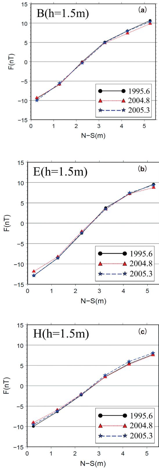
Fig.12 Total magnetic intensity measured in the absolute observation house along the north-south survey lines at 1.5 m above the floor. Black, red, and blue lines represent the first survey (June 1995), the second survey (August 2004), and the third survey (March 2005), respectively. Panels (a), (b), and (c) show measurements along survey lines B, E, and H, respectively.
